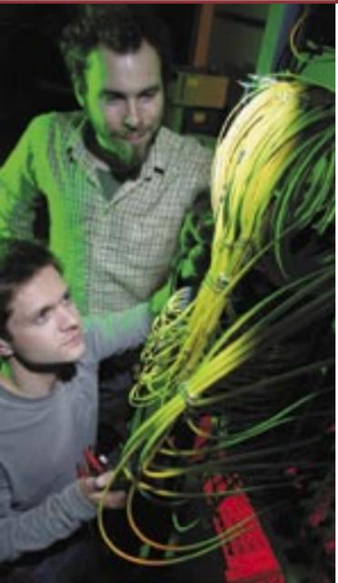
A researcher and a PhD student work together to cable and test some of the readout electronics of CMS.
