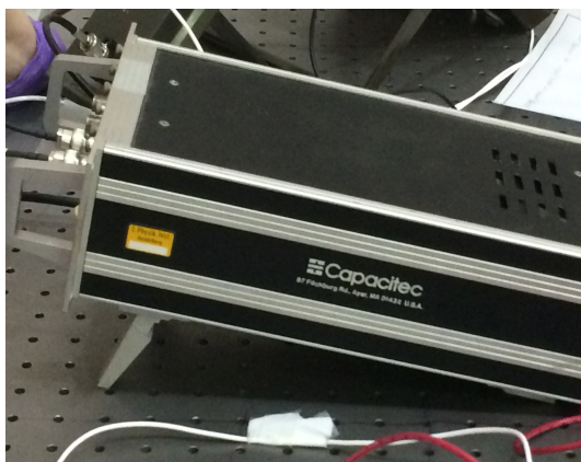
Figure 3.4: The Capacitec used for quad plate survey (left) and the calibration setting for recalibration (right).
