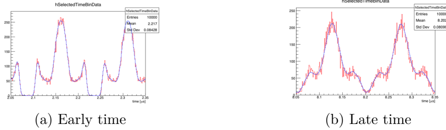
Figure 5.15: Example: gm2ringsim simulation results. Red: decay positron counts seen by calorimeters; Blue: expected counts from fast rotation analysis.
