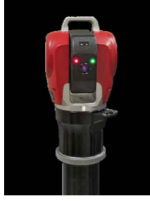
Figure 3.21: Laser alignment system for quad plate alignment.
