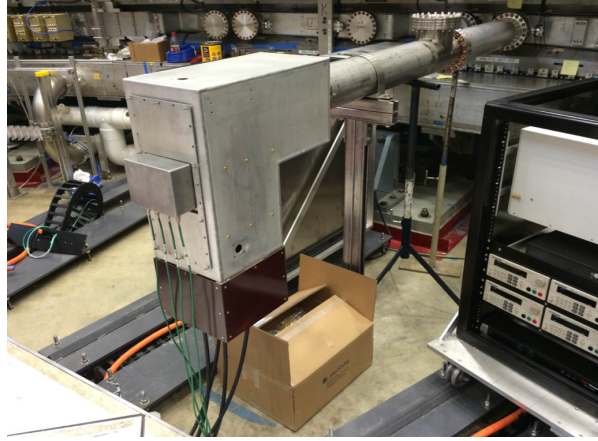
Figure 3.27: Example of a “successfully” installed quad extension.
