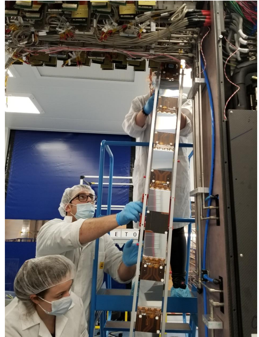
Upstream Tracker installations at CERN for the LHCb Upgrade (2022)
