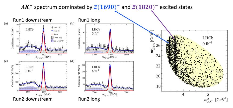
Long:  $\Lambda$  with a short flight distance that p and  $\pi$  have the decay vertex in the VELO (vertex detector) Downstream: p and  $\pi$  can't be formed in the VELO and are only reconstructed in the tracking stations
